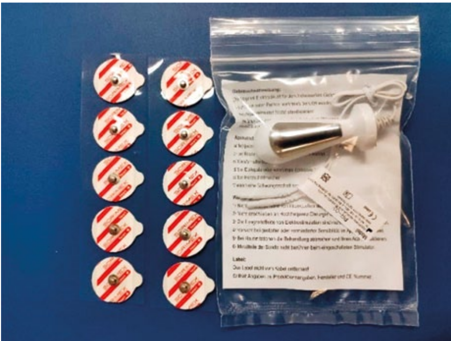
Figure 5. The endovaginal electrode and the surface electrodes used in the project (photographs: the author’s own material).
